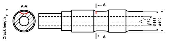
[Klinger C, Bettge D. Axle fracture of an ICE3 high speed train. Eng Fail Anal 2013;35:66–81. https://doi.org/10.1016/j.engfailanal.2012.11.008. http://eisenbahn.egghof.com/2008/11/ice-radsatzwellen-gedanken.html]
