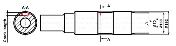
[Klinger C, Bettge D. Axle fracture of an ICE3 high speed train. Eng Fail Anal 2013;35:66–81. https://doi.org/10.1016/j.engfailanal.2012.11.008. http://eisenbahn.egghof.com/2008/11/ice-radsatzwellen-gedanken.html]
