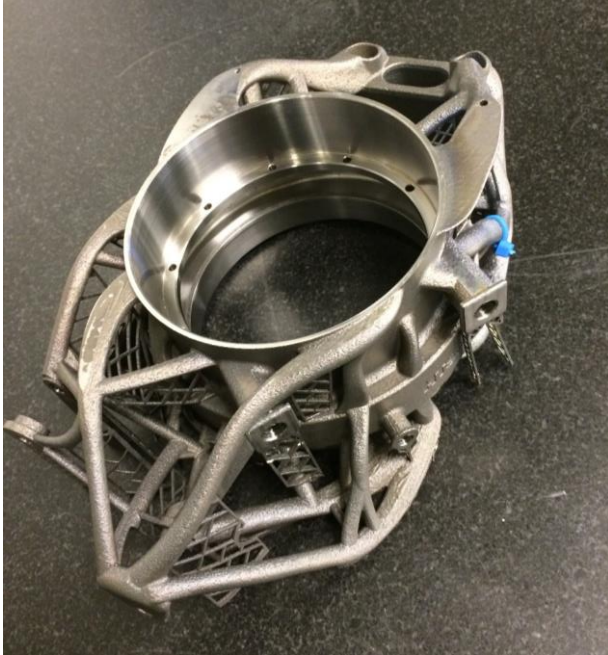
Front upright post CNC-machining
