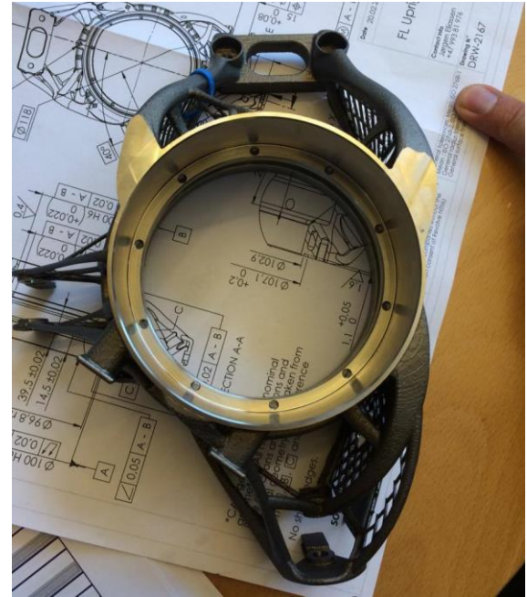
Rear upright post CNC-machining
