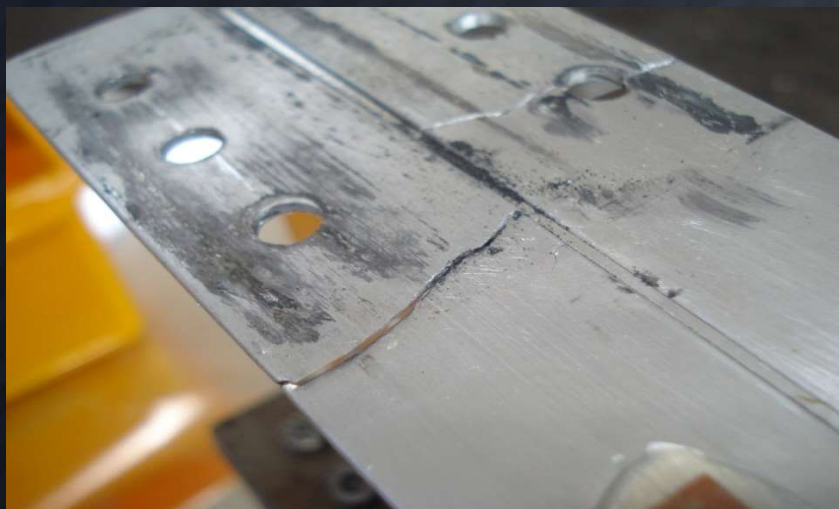
Real crack on the spar cap
