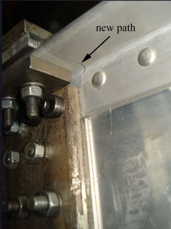
View of the crack on the cap (left) after stabilization (residual stress removal) and simulated crack path (right)
