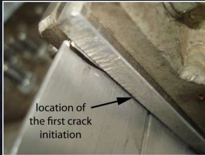
Locations and paths of cracks on horizontal walls of the spar caps
