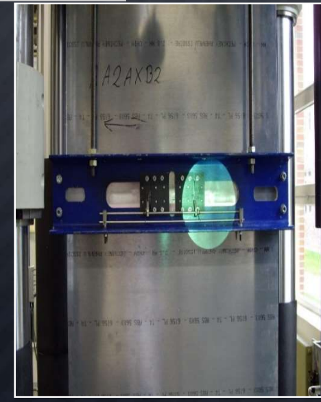
4-stringer panel (6156-T6) was tested in GKSS research center (Hamburg, Germany)
