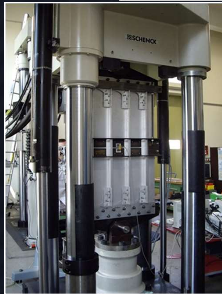
4-stringer panel (6156-T6) was tested in GKSS research center (Hamburg, Germany)
