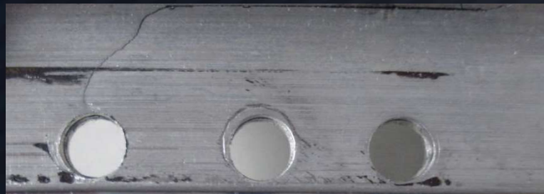
Cracks' growth paths on the vertical walls of the left and right spar cap
