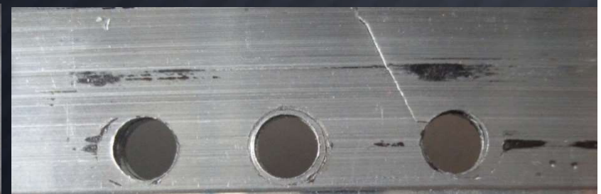
Cracks' growth paths on the vertical walls of the left and right spar cap
