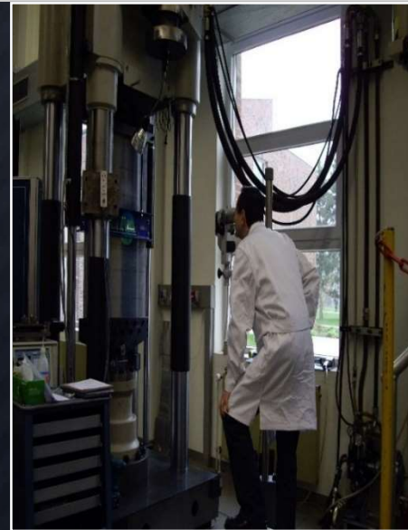
4-stringer panel (6156-T6) was tested in GKSS research center (Hamburg, Germany)
